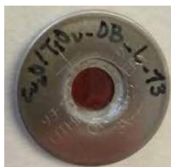
Figure 1. Photo of the photobattery consisting of an adapted coin cell.
