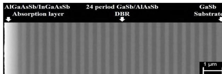
Figure 1. The cross-sectional scanning electron microscopy image of SESAM structure.
